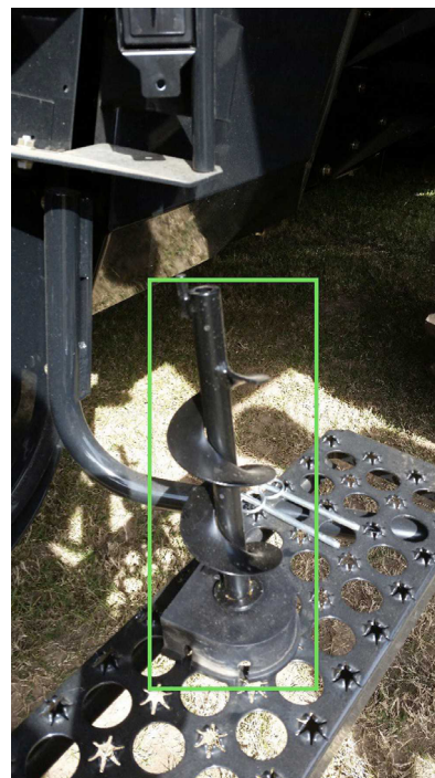
Figure 6. Small auger (inside green rectangle) for moisture sensor removed from cylinder container. Credits: Rebecca Barocco, UF/IFAS
