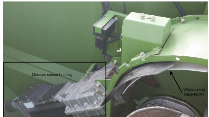
Figure 3. Curved impact-plate sensor (pointed by a black arrow) and moisture sensor housing (surrounded by a black rectangle) on the John Deere 9770 STS combine.
