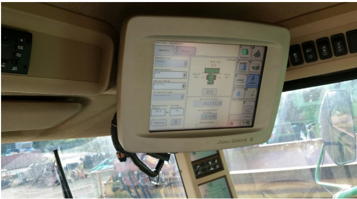
Figure 12. GreenStar™ 2 2600 computer display on the John Deere 9770 STS.
