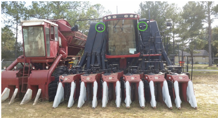
Figure 7. Location of optical sensor housing cut into the pneumatic ducts on a Case IH cotton picker (circled in green). Credits: Rebecca Barocco, UF/IFAS
