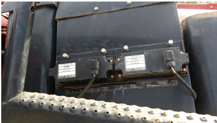
Figure 8. Close-up of optical sensor housing cut into the pneumatic ducts on a Case IH cotton picker. Credits: Rebecca Barocco, UF/IFAS
