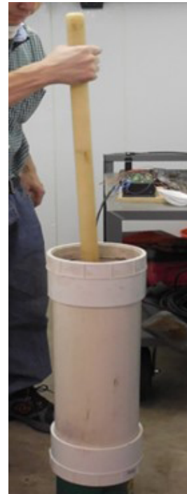
Figure 6. Compacting soil. Credits: Johanna Montanez, UF/IFAS
