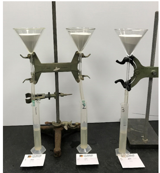
Figure 3. Laboratory experimental setup for measuring maximum water holding capacity.
