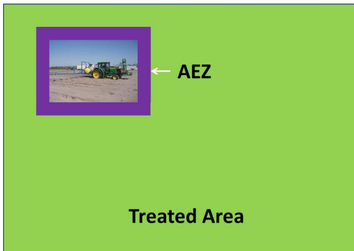
Figure 1. The AEZ is the purple area around the application equipment. It moves with the application equipment as it proceeds. The AEZ is generally within the treated area, except when the application equipment is near the edges of the treated area. Credits: Frederick Fishel, UF/IFAS
