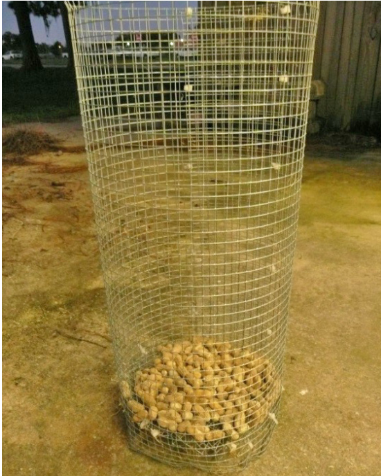
Figure 12. Hardware cloth basket designed to hold peanuts for blasting.
