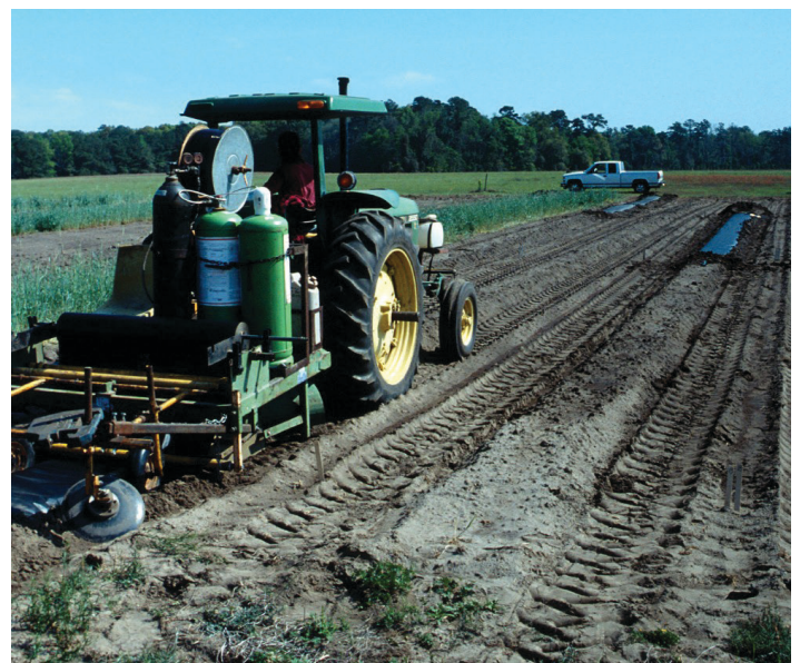
Figure 3. A combination mulch applicator that fumigates, presses the bed, and applies drip tape and plastic mulch in one pass.
