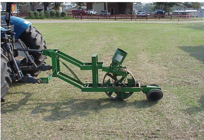
Figure 8. Planting unit for direct-seeding vegetables through polyethylene mulch.
