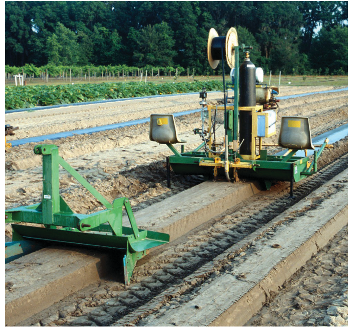
Figure 2. Bed press and mulch application machine (with drip tape attachment).
