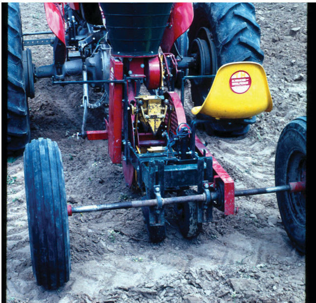
Figure 7. Direct-seeding through plastic mulch can be accomplished with this "plug-mix" planter. The machine punches a hole in the mulch and places a small amount of "soiless" mixture and seed into the hole.
