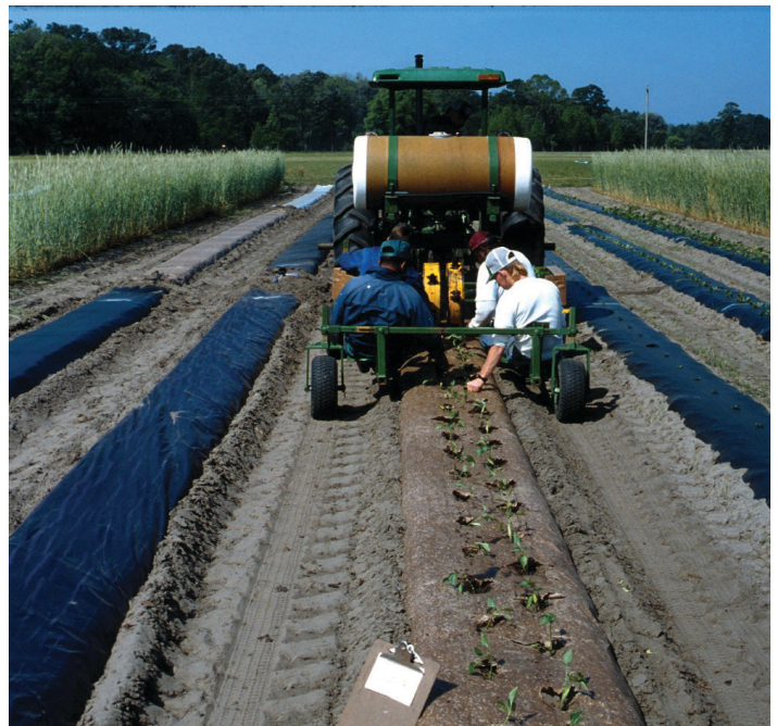
Figure 5. A water-wheel transplanter such as this one in use at Live Oak can place plants at various spacing and apply water or fertilizer solution with the plants.
