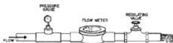
Figure 2. Pump capacity measuring apparatus, including a pressure gauge, flow meter, and regulating valve.
