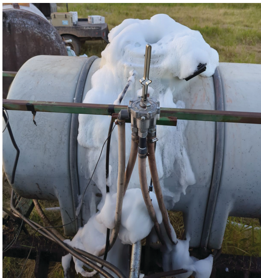
Figure 4. Excessive foaming from improper mixing order, excessive agitation, or pesticide incompatibility. Foaming can also increase pressure and damage equipment.
