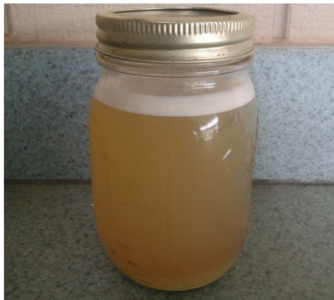
Figure 6. After mixing and allowing the jar test time, settling has occurred. This could indicate incompatible pesticides or a need for constant agitation. The top layer is solid and will no longer mix, indicative of incompatibility.
