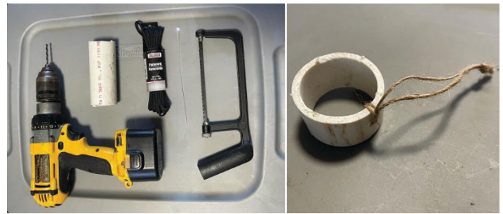
Figure 4. DIY scallop sorter using a PVC ring (two inches or larger) to support the scallop population.
