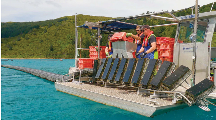
Figure 5. FlipFarm Systems Ltd using the “flipper” to fill baskets with oysters for growout.
