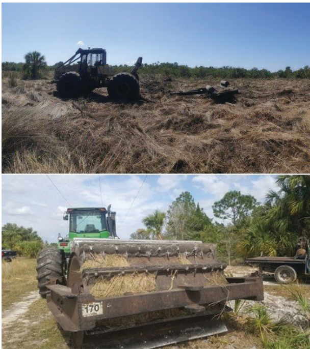
Figure 1. Common roller chopper setups. Credits: Top—Amy Copeland, St. Johns River Water Management District; Bottom—Graham Williams St. Johns River Water Management District. All images used with permission.
