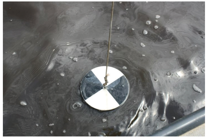
Figure 1. A Secchi disk is a black and white circular disk used to measure water clarity. The disk is slowly lowered into the water until it is no longer visible. It is then slowly raised until it becomes visible again. The depth when the disk first becomes visible is then measured and referred to as “Secchi depth.” Higher Secchi depth values indicate clearer water.
