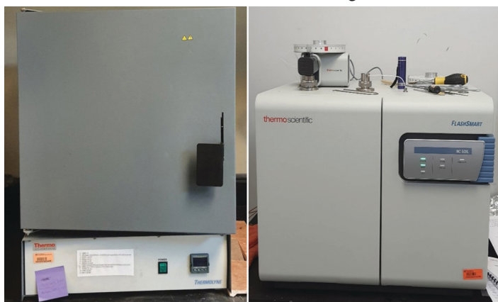
Figure 2. Incinerator for measuring C (left) and Dry Combustion Elemental C Analyzer (right).
