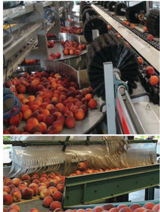
Figure 6-8. Counter directional soft bristle brushes (above) and plastic curtains (below) are used to decelerate peaches to reduce mechanical damage on the packingline. Credits: Mark A. Ritenour, UF/IFAS
