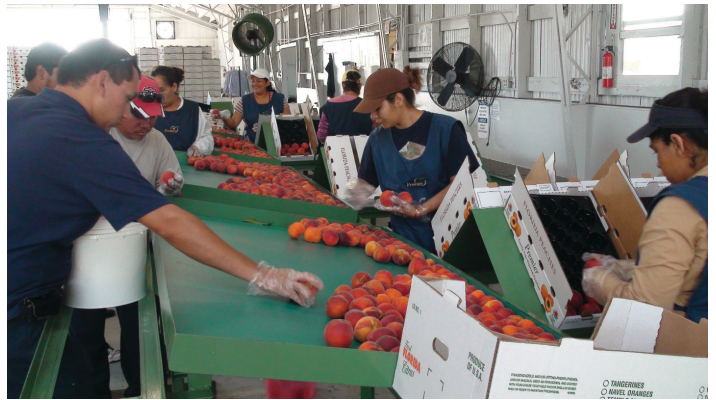
Figure 6-22. Combined grading and packing of fruit from buckets into trays at a ranch pack operation.
