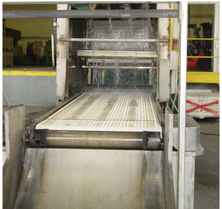
Figure 6-17. Washing system for field bins. Credits: Mark A. Ritenour, UF/IFAS
