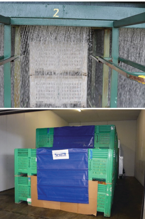
Figure 6-5. Top, a bin hydrocooler and bottom, a forced-air cooler. Credits: Jeffrey K. Brecht, UF/IFAS
