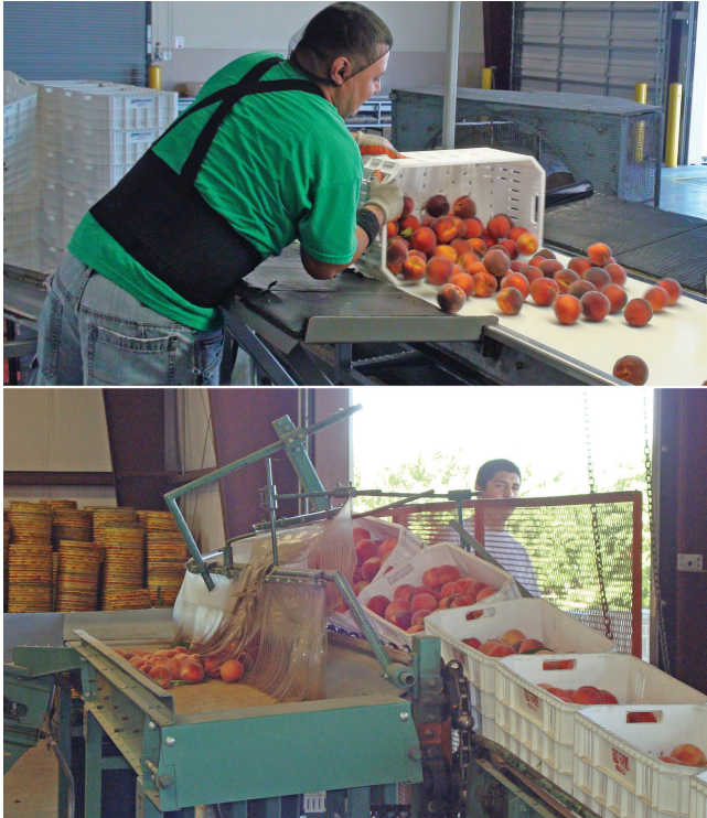
Figure 6-7. Manual (above) and automated (below) dumping of peaches from field boxes onto the packingline. Credits: Mark A. Ritenour, UF/IFAS
