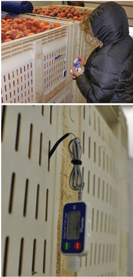
Figure 8-3. Probing fruit during cooling assures that the final temperature is reached. Here, a datalogger with its temperature probe is placed into a peach fruit during forced-air cooling. Credits: Jeffrey K. Brecht, UF/IFAS
