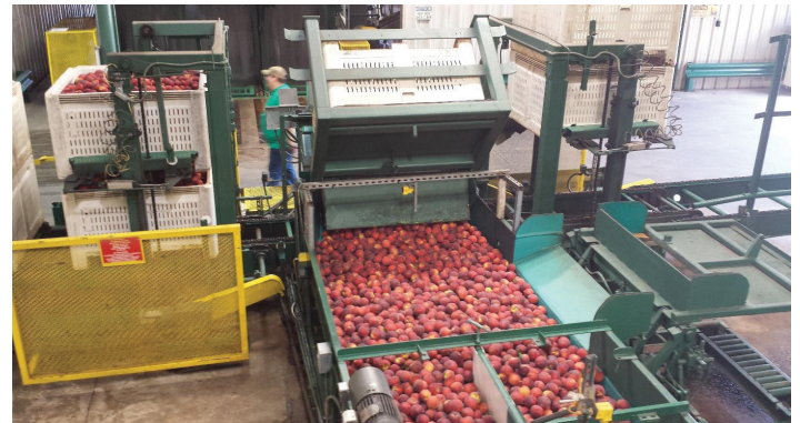
Figure 6-6. Bin dump. Stored peaches taken from the cold room (rear) and transferred from filled bins onto the packingline. Credits: Jeffrey K. Brecht, UF/IFAS
