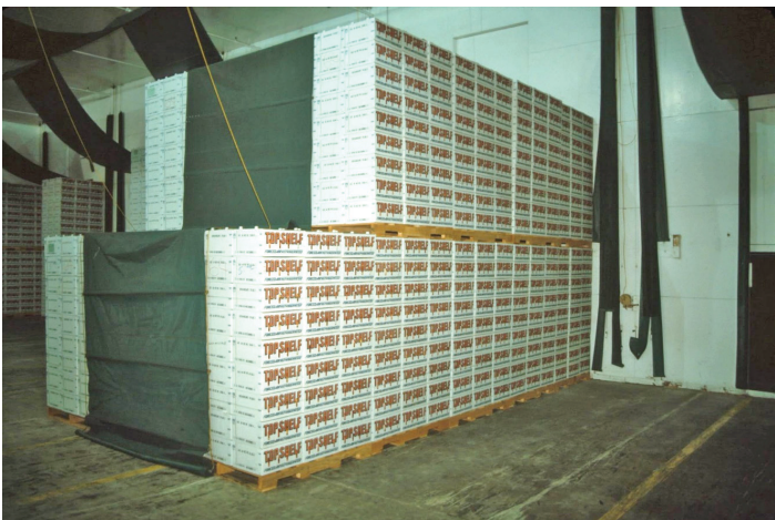
Figure 6-16. Forced-air cooling of palletized product. Credits: Mark A. Ritenour, UF/IFAS
