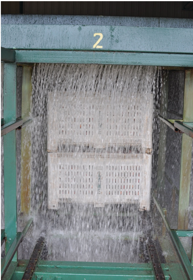
Figure 8-9. A continuous or tunnel hydrocooler in which the conveyor speed determines the duration of cooling.
