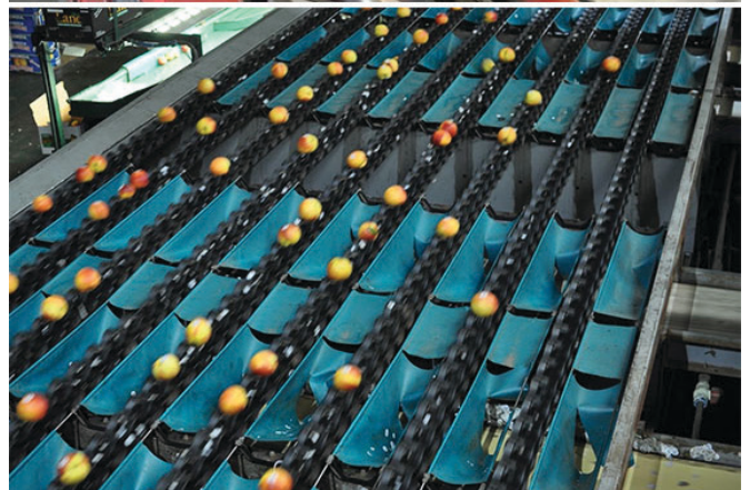
Figure 6-12. Fruit sizing being accomplished by a camera system (above) and a weight sizer (below). Credits: Jeffrey K. Brecht, UF/IFAS
