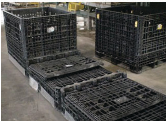
Figure 5-11. Top, plastic field bin. Bottom, plastic bins that can be collapsed to conserve space during transport and storage between uses.
