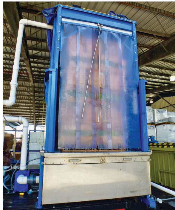
Figure 8-8. A stationary (batch) hydrocooler, which runs for a predetermined time to achieve 7/8 cooling. Credits: Jeffrey K. Brecht, UF/IFAS
