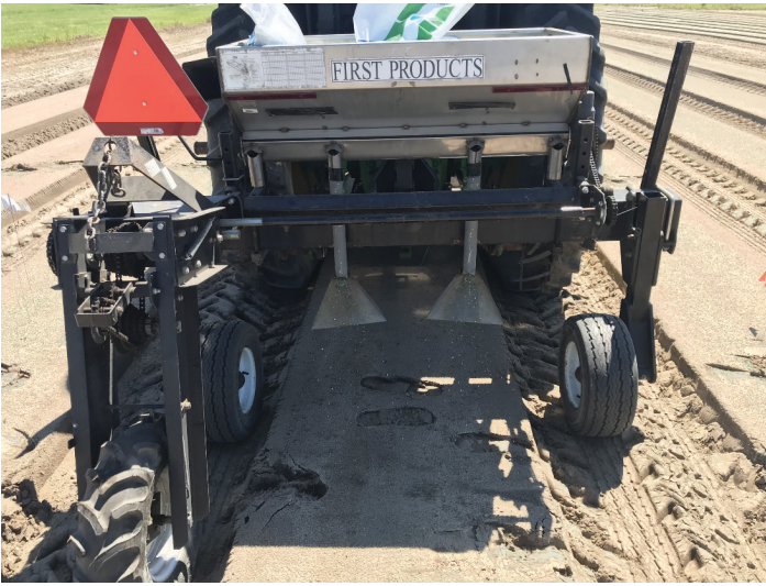
Figure 8. Fertilizer application using a drop spreader to uniformly apply the fertilizer across the bed top.
