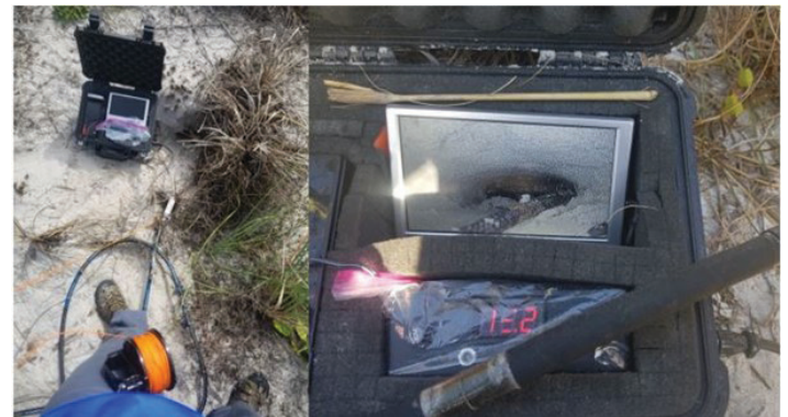
Figure 14. Gopher tortoise burrow scope used for determining occupancy of burrows (iguana tail visible on monitor). Credits: Sean L. McKnight, UF/IFAS
