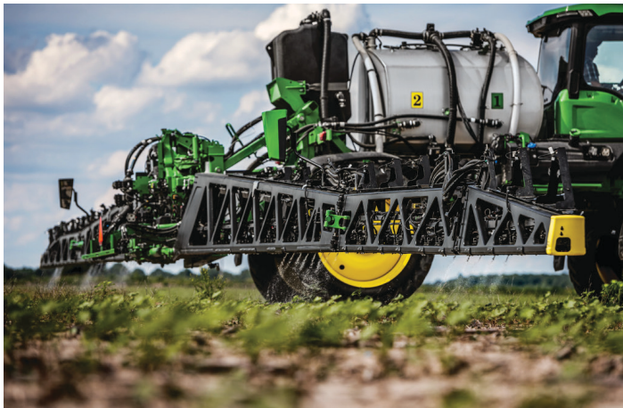
Figure 4. Computer vision system for target spraying for weeds. The sprayer is equipped with 36 cameras and machine learning algorithms to detect weeds among corn, soybean, and cotton plants. Credits: John Deere, used here under Creative Commons license CC BY 2.0. Source: https://www.flickr.com/photos/32295574@N05/52201229970
