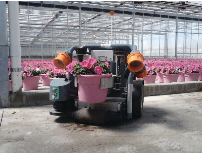
Figure 6. A snapshot of HV-100 Robot for spacing (square or hex pattern) and collection of potted plants for labor-saving, increased plant health, and energy efficiency.
