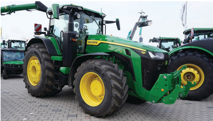
Figure 7. John Deere's new 8R tractor series for fully autonomous driving and tillage. John Deere announced earlier in 2022 that they were preparing for large-scale production of the autonomous tractor. The 8R tractor uses six pairs of stereo vision (3D perception) and AI to navigate and plow the soil and sow seeds autonomously.
