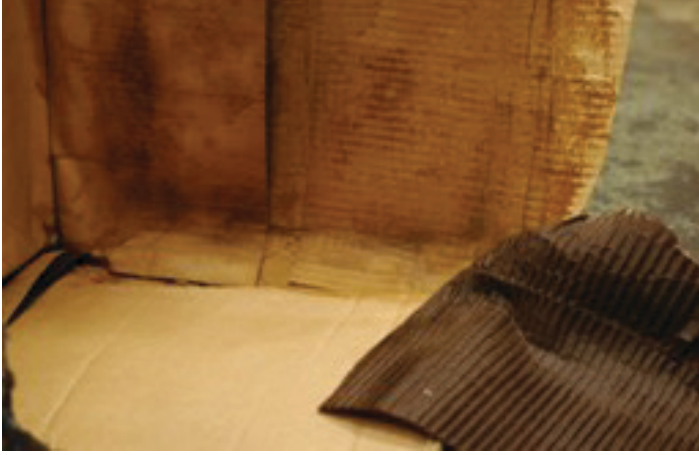
Figure 2. Leaking box. The primary and secondary packaging were not leakproof. Absorbent material was not included to absorb the contents.
