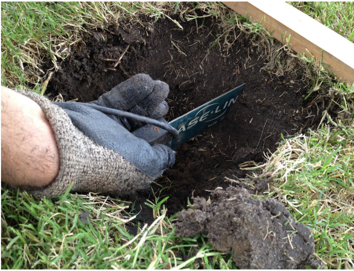
Figure 1. An example of a soil moisture sensor being installed in the soil. Credits: Michael Gutierrez, UF/IFAS
