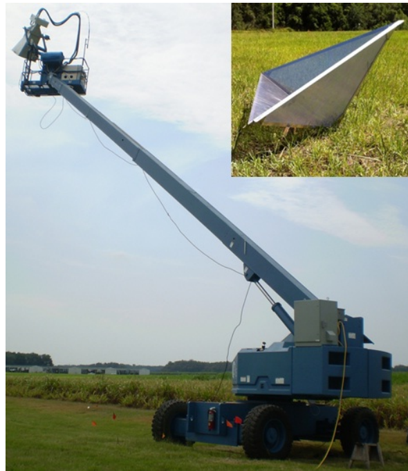
Figure 9. UF-LARS mounted on the 25 m Genie platform. (Inset) Trihedral calibration target made of aluminum with an aperture length of 1.28 m Credits: Nagarajan et al. (2014)
