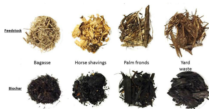
Figure 3. Four feedstocks converted to biochar using the TLUD gasifier.
