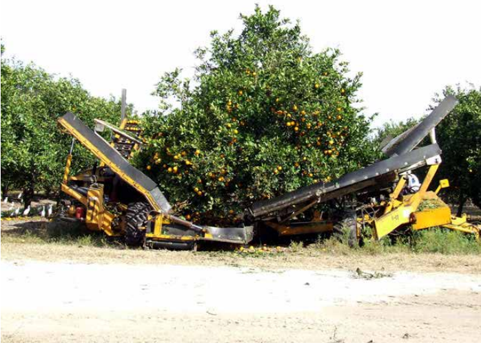
Figure 5. A Coe-Collier system harvesting a tree with the two-system shaker and receiver units (Photo courtesy of Barbara Hyman, UF/IFAS)
