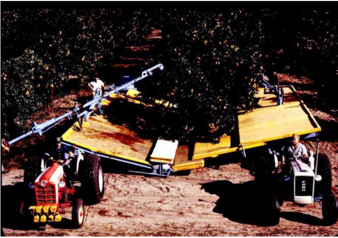
Figure 1. Early version of a citrus trunk shaker (Photo courtesy of Dr. Jodie Whitney, UF/IFAS)
