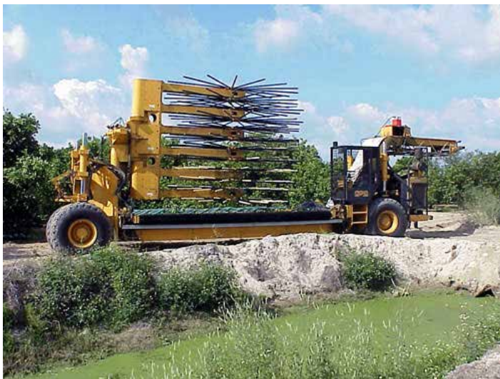
Figure 1. Continuous canopy shake and catch (CSC) system, Oxbo Freedom 3220 (Photo courtesy of Barbara Hyman, UF/IFAS)
