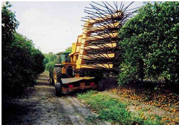
Figure 3. Tractor-drawn continuous canopy shaker (TD-CS) system, Oxbo 3210 (Photo courtesy of Barbara Hyman, UF/IFAS)
