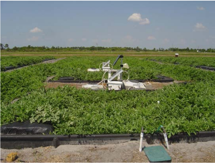
Figure 1. The drainage lysimeter for the watermelon crop water-use experiment
