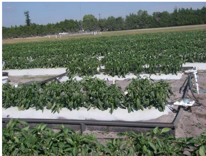
Figure 1. The drainage lysimeter for the pepper crop water-use experiment
