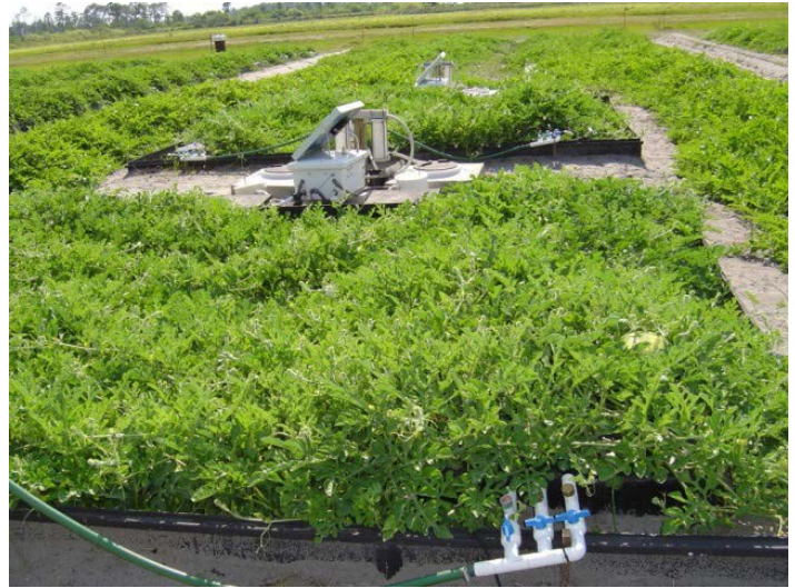
Figure 1. The drainage lysimeter for watermelon experiment Credits: Sanjay Shukla
