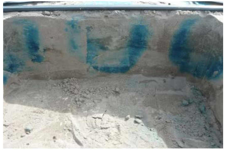
Figure 4. Wetting width along the bed Credits: Holt and Shukla
