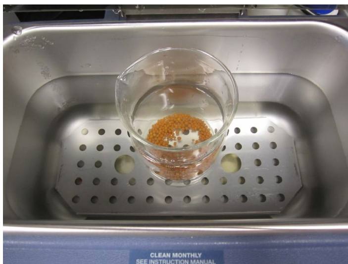
Figure 2. Standard temperature-controlled incubation of 0.44 oz of CRF in 8.4 fl oz water incubated at 77 °F
