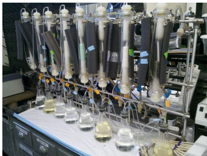
Figure 3. An accelerated temperature controlled incubation unit as described by Sartain et al. (2004).
