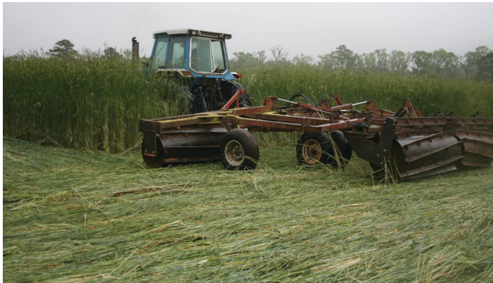
Figure 2. Terminating a high-residue cereal rye cover crop using a roller-crimper.
