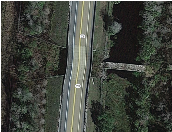
Figure 7. An example of a wildlife crossing on CR 29 in south Florida. Wildlife fencing funnels wildlife to a bridged underpass area where it connects to a wildlife bridge. Click this link to see photos and videos of wildlife using these structures.
