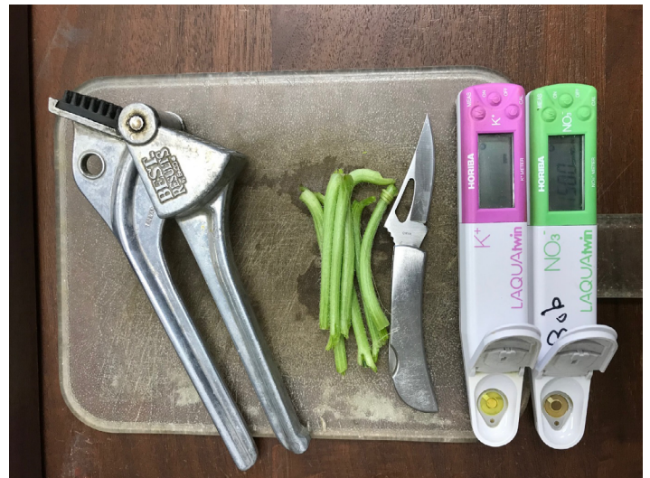
Figure 5. Horiba LAQUA twin meters for Nitrate-N and K with sample. Credits: Robert Hochmuth, UF/IFAS
