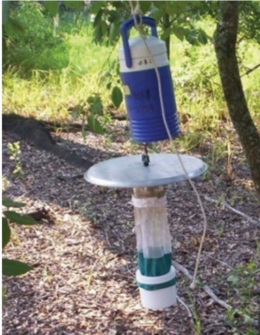
Figure 8. A CDC miniature light trap with a cooler containing dry ice hanging above it.
