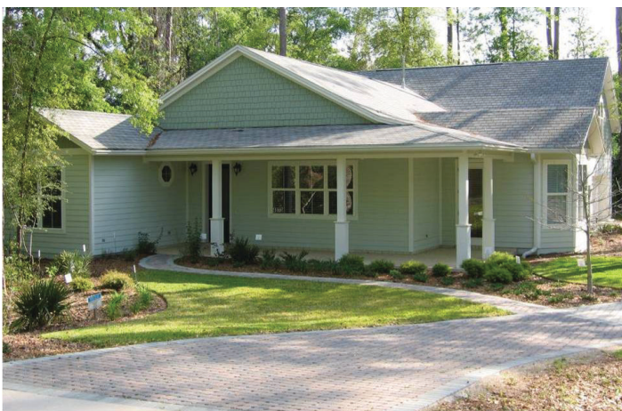
Figure 4. Another Gainesville, Florida home with more natural landscaping. It has a small patch of lawn, a natural landscaped rain garden, conserved trees, and a permeable paved driveway.
