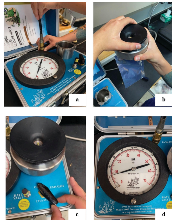
Figure 5. Steps (a–d) for measuring leaf water potential using the pressure “bomb” method.
