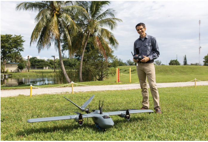
Figure 3. Example of a hybrid VTOL UAV. Credits: UF/IFAS
