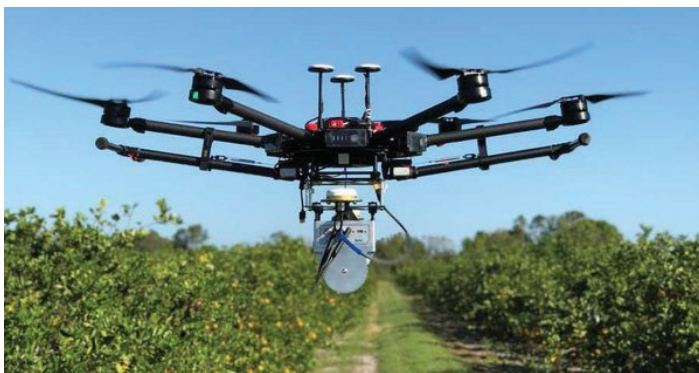
Figure 6. UAV equipped with a LiDAR mapping system. Credits: UF/IFAS
