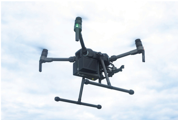
Figure 1. Example of a multi-rotor UAV (Matrice 210 from DJI, Shenzhen, China). Credits: UF/IFAS
