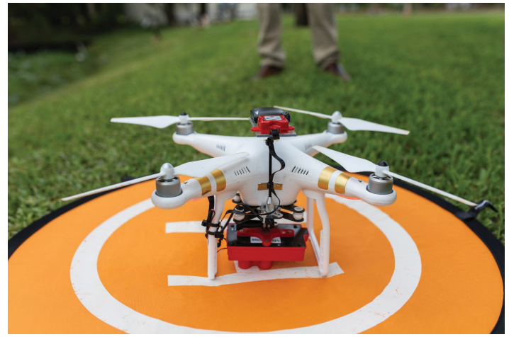
Figure 4. UAV equipped with a multispectral sensor (Altum, RedEdge-M, AgEagle Aerial Systems Inc., Wichita, KS, US). Credits: UF/IFAS
