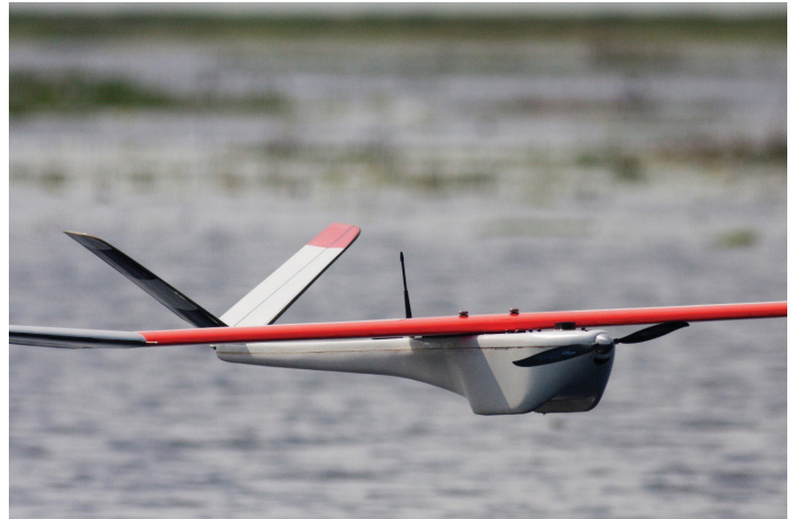
Figure 2. Example of a fixed-wing UAV (created by UF researchers, Gainesville, FL, US). Credits: UF/IFAS
