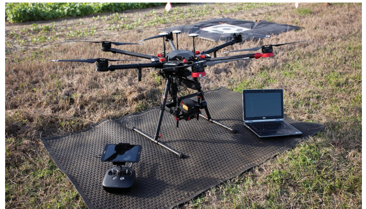
Figure 5. UAV equipped with a hyperspectral sensor. Credits: UF/IFAS
