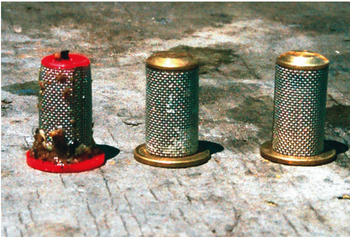
Figure 1. Debris-clogged nozzle tip screens (left and center); clean screen (right).
