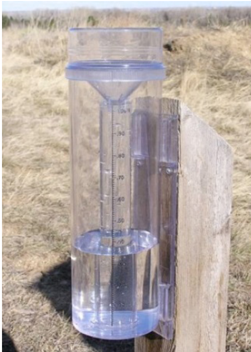
Figure 2. Manual rain gauge from the Community Collaborative Rain, Hail & Snow Network (CoCoRAHS) Credits: CoCoRAHS
