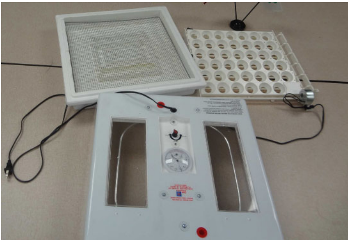
Figure 3. A still air incubator and an automatic egg turner Credits: Marcus Boston, UF/IFAS
