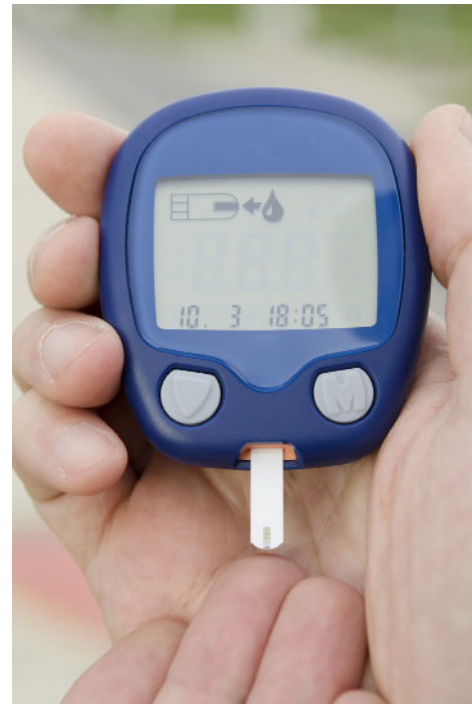
Figure 1. A blood glucose meter (or glucometer) uses a tiny drop of blood to test your blood glucose level.
