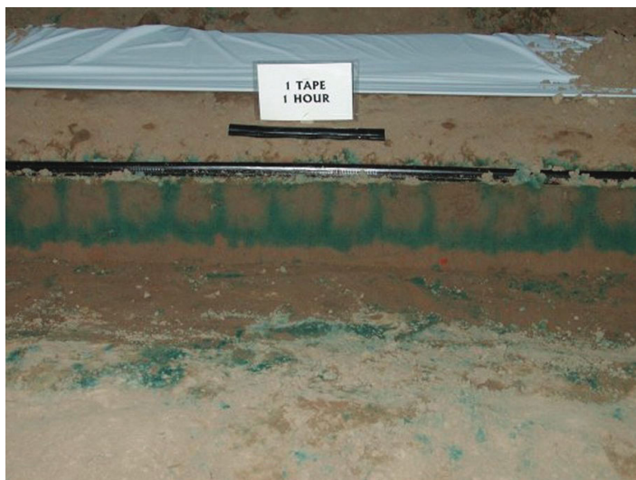
Figure 4. Soluble blue dye may be used to visualize wetting patterns and understand how irrigation volume affects water movement in the bed. For short irrigation times (1 hour) a more even water distribution pattern may be expected with a 4-in emitter spacing (4.1) than with an 12-in emitter spacing (4.2). Flow rates were 33 gal/100 ft/hr for the 4-in emitter spacing, and 30 gal/100ft/hr for the 12-in emitter spacing. The presence of an impermeable clay layer at the 10-in depth (in Gadsden county) resulted in lateral movement as shown in (4.3) where the blue dye is in the alley (between the 3 rd and 4 th bed from the right) after 6 hours of irrigation delivering 180 gal/100ft. The presence of water and soluble nutrients in the row middles will likely promote weed growth. Wetting patterns in the very compacted beds used for strawberry production in Hillsborough county are rectangular which corresponds to an increase in lateral water movement as shown in (4.4) after a 6-hr irrigation that delivered 144 gal/100 ft with a 12-in emitter spacing.
