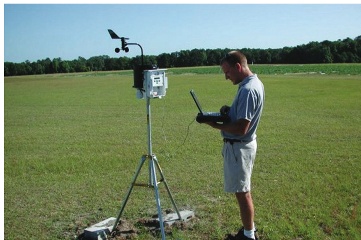
Figure 3. Tools and techniques available to estimate evapotranspiration and irrigation needs: (3.1) weather data may be simply downloaded from a small automated weather station to calculate reference evapotranspiration (ET o ) and (3.2) water loss in the reservoir of the atmometer mimics ET o .
