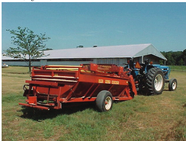
Figure 9. Manure spreader that can be used to apply manure for mulched vegetable crop production. Credits: J. Jones
