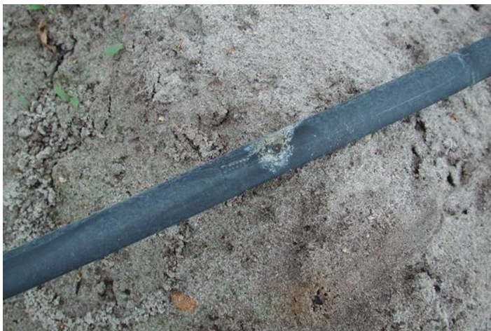
Figure 7. Accumulation of precipitates around a drip-tape emitter (8.1) may result in an uneven water distribution pattern (8.2).
