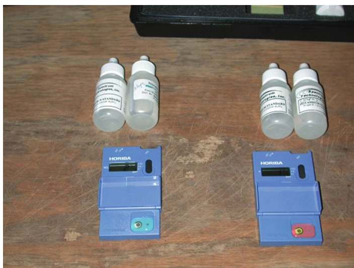
Figure 2. Sap testing for vegetables involves separating the petiole from the leaf blade, (2.1) calibrating the nitrate (NO 3 -N) and potassium (K) ion specific electrodes (Cardi meter shown here) with standard solutions, (2.2) extracting the sap, (2.3) collecting the sap from the press, and (2.4) placing a droplet of sap on the electrode. A hydraulic press may be needed only when few petioles are available or when petioles contain little sap as may occur with strawberry. In most cases, a garlic press will be an adequate tool to extract the sap. Readings should be compared to published sufficiency ranges.
