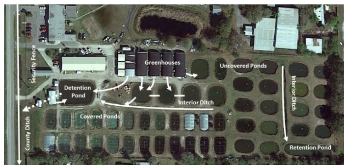
Figure 1. Representative fish farm layout showing several structural barriers used to prevent the release of organisms. Visible structural strategies include covers on ponds, a detention and retention pond, and a security fence surrounding the property. Further, riser-board control structures are found on both interior ditches before they flow to the detention or retention pond. Screening is also present on all vats and aquaria in the greenhouses. Water-flow direction is indicated by arrows.
