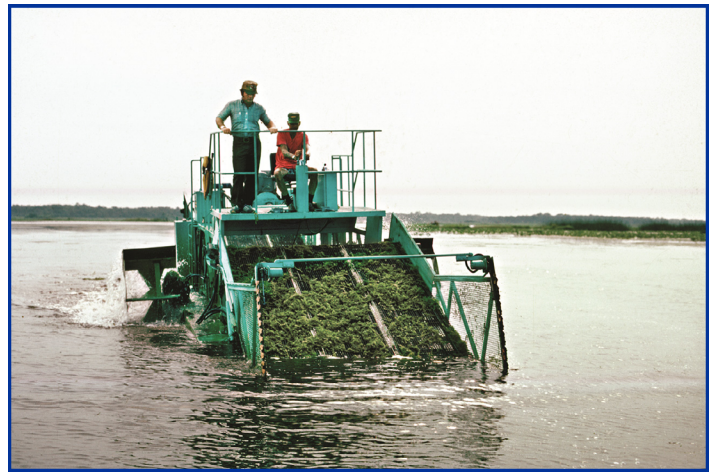
Figure 7. Mechanical harvesting of hydrilla. Credits: Bill Haller.
