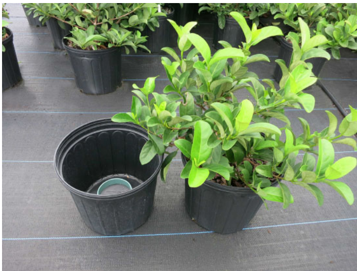
Figure 2. Containers of sprinkler-irrigated plants are placed inside similar-sized holeless containers to collect leachate (drainage) during LF testing. A PVC ring or other object that elevates the plant container is placed at the bottom of the holeless container to allow drainage to occur without reabsorption. We recommend using holeless containers obtained from the manufacturer for routine LF testing due to simplicity and speed of setup.
