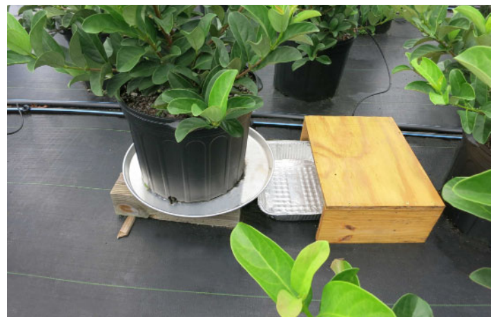
Figure 3. Micro-irrigated plants can be placed on a pan raised several inches off the ground with pieces of 4"x4" lumber. A drain hole punched out of the pizza pan allows leachate to drain into an aluminum tray for easy measurement. An emitter from an adjacent container is placed in a pail to determine the irrigation amount. This setup can remain in the field to facilitate routine testing. We often place a cover over the tray when collecting leachate during multiple irrigation cycles.
