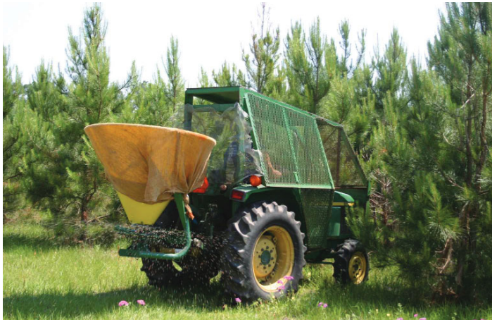
Figure 2. Mineral fertilizer application with a centrifugal fertilizer spreader. Note the cage on the tractor and the cover on the spreader, especially useful in younger stands.
