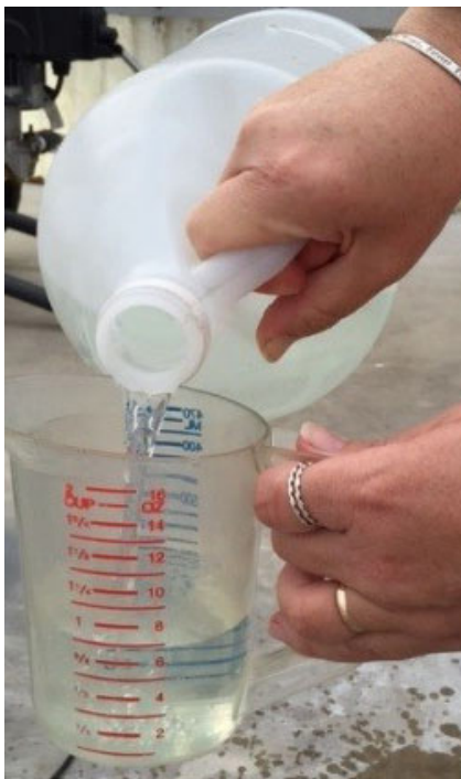
Figure 9. Measuring leachate volume. Credits: UF/IFAS
