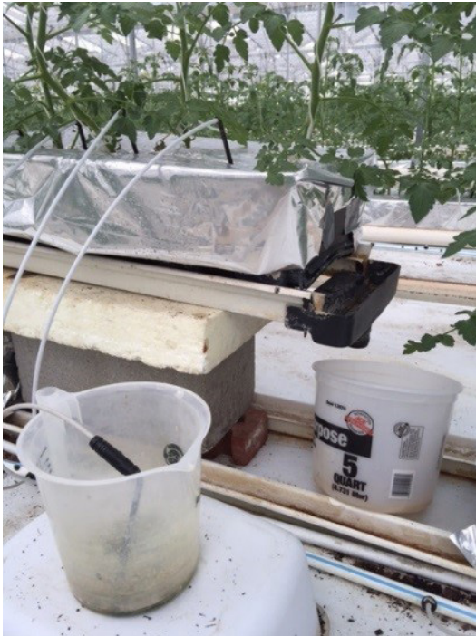
Figure 3. Leach collection system in a commercial greenhouse. Credits: UF/IFAS
