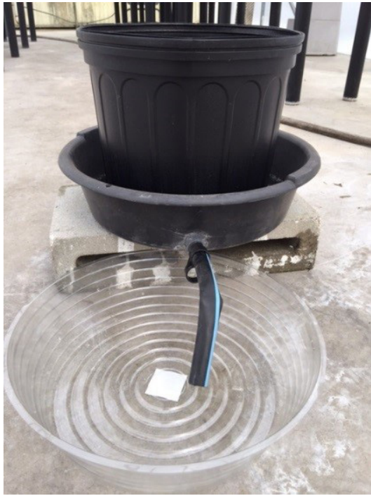
Figure 5. Using an oil pan drain to catch leachate. Credits: UF/IFAS
