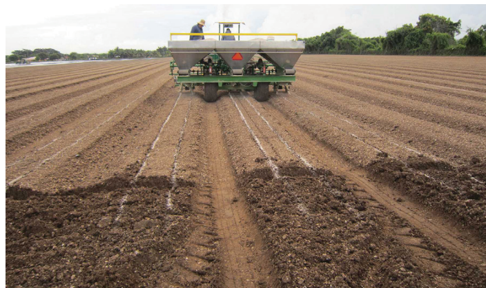
Figure 5. Pre-plant application of a conventional fertilizer 6-6-12 (N-P 2 O 5 -K 2 O) in percentage with a rate of 1,200 lb per acre on raised beds. Credits: Qingren Wang, UF/IFAS
