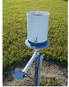
Figure 1. Tipping bucket rain gauge. Credits: K. W. Migliaccio, UF/IFAS
