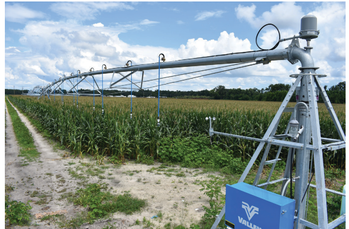
Figure 1. Center pivot irrigation system with low pressure drop nozzles increase crop water uptake efficiency. Credits: Charles Barrett, UF/IFAS
