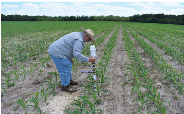
Figure 2. Joel Love, BMP outreach specialist, installs a soil moisture sensor for a corn grower.
