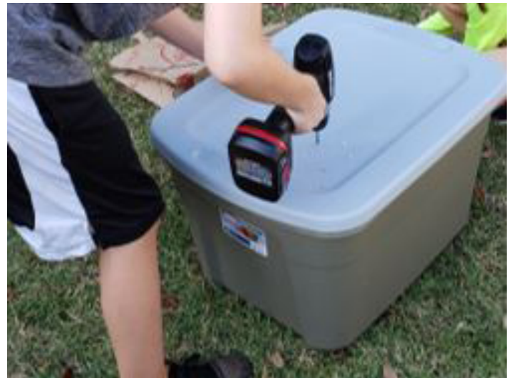
Figure 9. Single worm bin assembly. Step 1: Drill holes in lid and bottom of upper bin.
