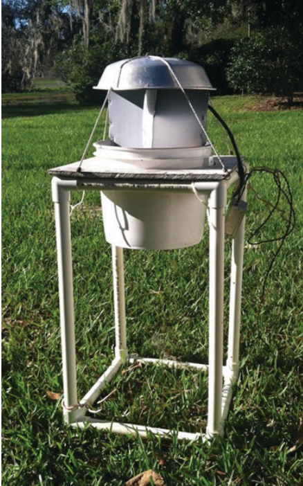
Figure 6. Black light trap for attracting and collecting click beetle adults at night. The electric light attracts adult click beetles, and a funnel below directs them into the bucket. Credits: R. Hochmuth, UF/IFAS
